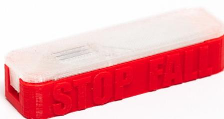
Stop Fall module is designed to detect whenever your UAV begins to fall and to automatically activate safety system. Internal sensor continuously measures the speed and the position and once UAV will start falling Stop Fall will send a signal to deploy the parachute. Along with automatic crash detection Stop Fall is able to use incoming PWM signal from flight controller or a receiver to let you activate the parachute manually.
